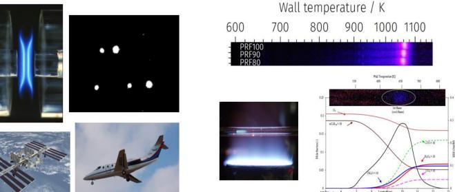
Some images of Microgravity program (conventional counterflow flame, flame balls) and Micro Flow Reactor (Weak flames for PRF 80-100, stabilized cool flame of n-heptane/air mixture)
