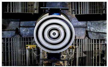
The X3 is a three-channel nested Hall thruster built at PEPL in collaboration with NASA JPL and AFRL, and is designed to operate at up to 200 kW of discharge power. This project is currently funded by the NASA NextSTEP initiative for the development of 100 kW class electric propulsion devices in support of manned Mars exploration.
