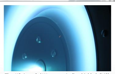
The H9 is a 9 kW magnetically shielded (MS) laboratory Hall thruster built in a collaboration between PEPL, NASA JPL, and AFRL, and is a common test platform for experiments on MS Hall thrusters. This close up image shows the efficient shielding of the discharge chamber walls from the plasma for erosion mitigation
