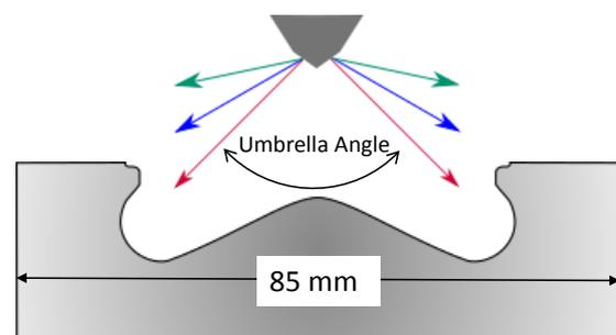
Figure 1. Piston head bowl and spray trajectories for 90° (red), 120° (blue), 156° (green) umbrella angles.
