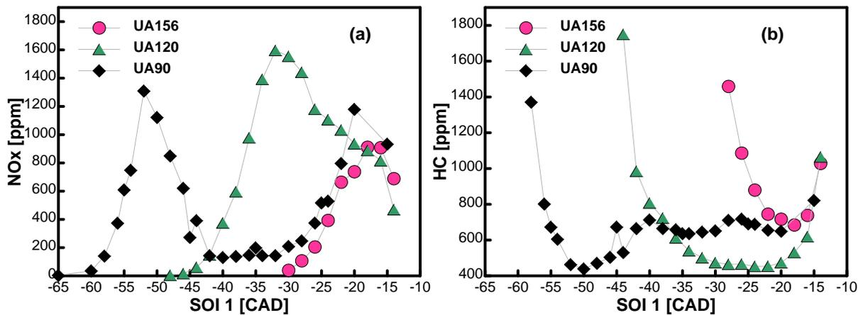
Figure 3 NOx emission and HC emissions as a function of the Injection Timing for different umbrella angles.
