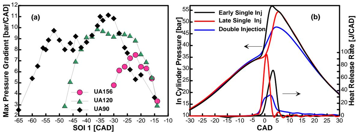
Figure 5: Max Pressure Gradient as a function of SOI (a). In-Cylinder Pressure and Heat Release Traces For Single Injection at SOI=-55CAD (Black Lines), Single Injection at SOI = -26 CAD (Red Lines) and for a Double Injection (Blue Lines).
