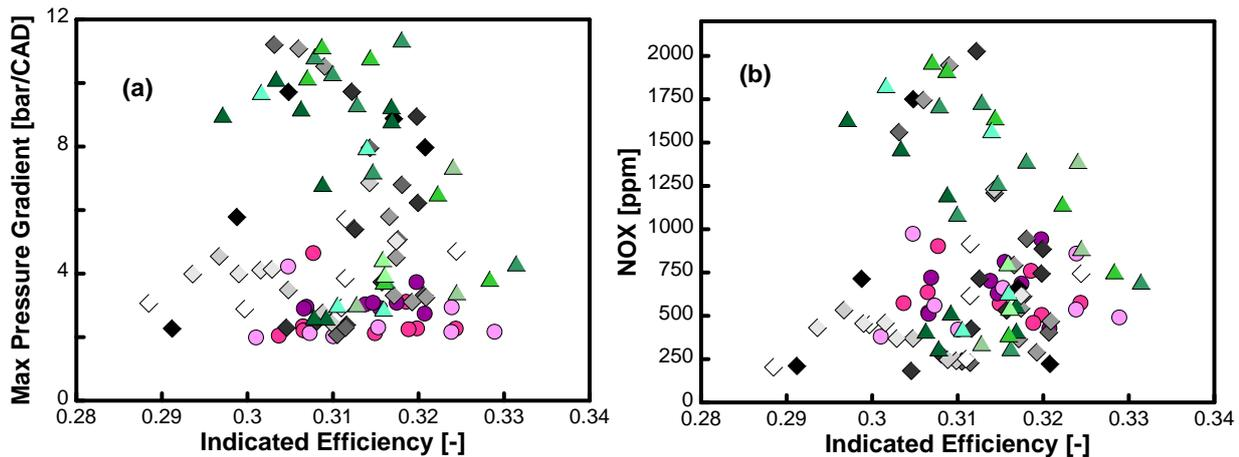
Figure 7: Max Pressure Gradient as a function of Indicated Efficiency (a). NOx emission as a function of Indicated Efficiency. Double Injection strategy for each of the injector tested.
