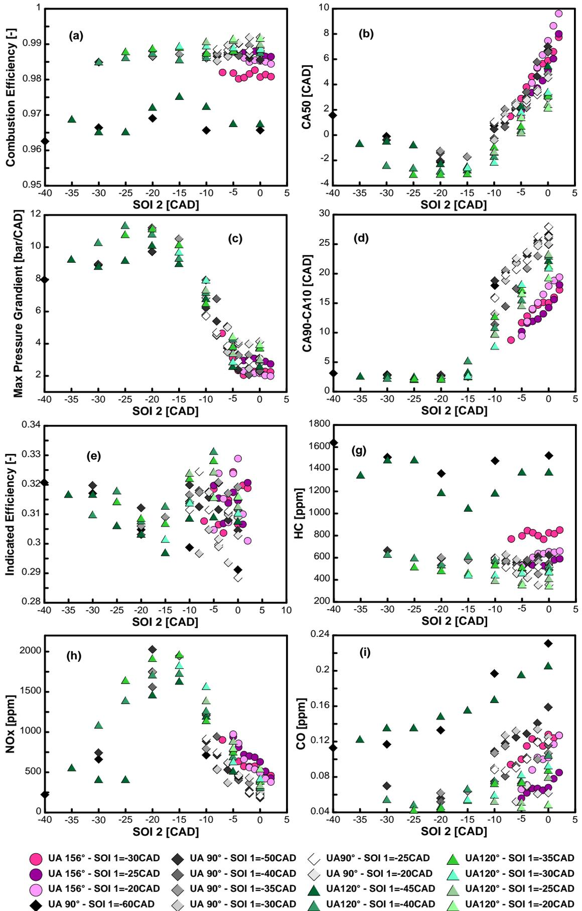
Figure 4 Combustion Parameters and Pollutant Emissions as a function of SOI1 and SOI2
