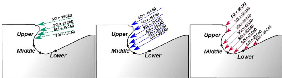
Figure 4: Spray target position as a function of SOI for the UA156, UA120 and UA90 injectors.
