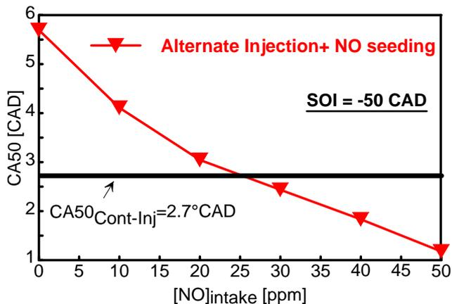
Figure 7 Evaluation of the NO trapped fraction. CA50 as a function of NO concentration, during alternate-fired mode.
