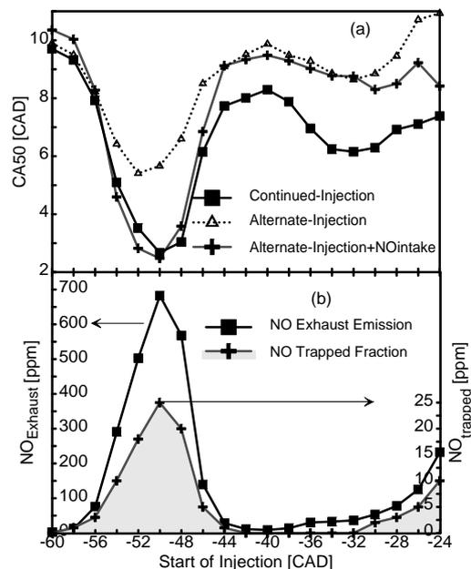
Figure 6 CA50 as a function of SOI for the continued-injection mode, alternate-injection mode and alternate-injection mode with NO addition at the intake (a). Exhaust NO concentration measured in the continued-injection mode and the estimated NO trapped fraction
