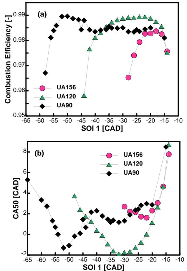
Figure 2 Combustion Efficiency and Combustion Phasing as a function of the Injection Timing for different umbrella angles
