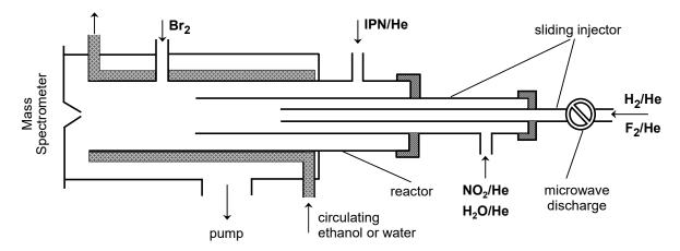
Figure 1 Diagram of the flow reactor.
